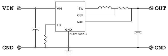
Note: When using a solid or ceramic input Cap, It is recommended to parallel a TVS diode.
