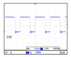
Fig 4 SW Waveform
