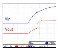
Fig 3 Startup with Vin
