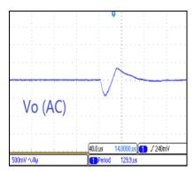
Fig 5 Transient Response (V<sub>IN</sub>=3.6V, Vout=5V, I<sub>load</sub>=0.15A to 0.9A)
