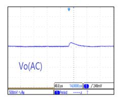
Fig 6 Transient Response (V<sub>IN</sub>=3.6V, Vout=5V, I<sub>load</sub>=0.9A to 0.15A)
