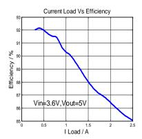
Fig 2 Efficiency Vs Heavy Load
