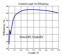
Fig 1 Efficiency Vs Light Load
