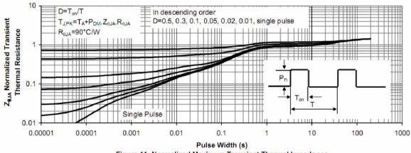
Figure 11: Normalized Maximum Transient Thermal Impedance
