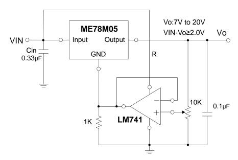
The addition of an operational amplifier allows adjustment to higher or intermediate values while retaining regulation characteristics. The minimum voltage obtainable with this arrangement is 2.0 V greater than the regulator voltage.
