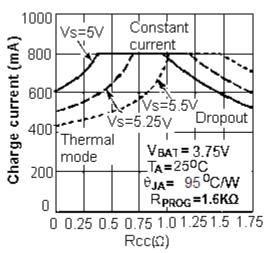
Fig.4:The relationship curve between charge current with R<sub>CC</sub>
