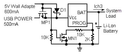
Fig.5:Combining Wall Adapter and USB Power
