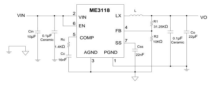
Fig.1 3.3 V 3 A Synchronous Buck Regulator, Fs = 500 KHz
